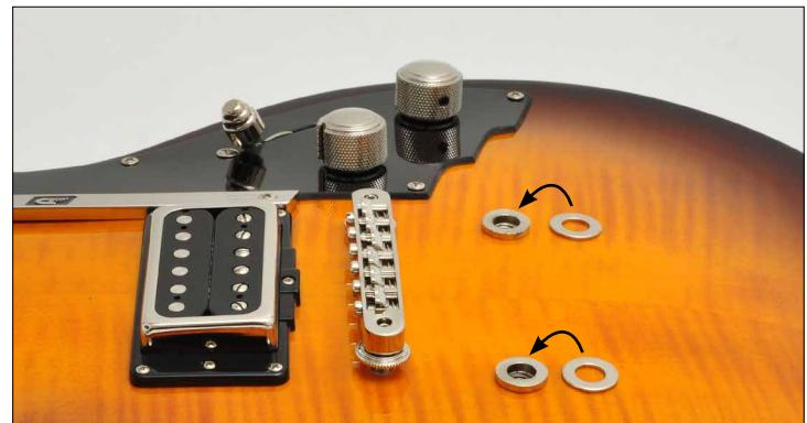
Now carefully place the **göldo LT tremolo** onto the top of the anchor bushings. The tremolo should not rest on the top of the guitar. If it does, simply place one or two of the enclosed washers between the bushings and the tremolo before mounting.
